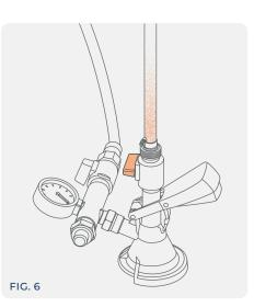
Work with the product valve to remove any residual gas from the product tube. Close the product valve.
