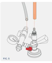
K-VALVE ONLY Connect the product and gas tubes to the filling kit. Open the red valve.
