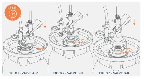
Make sure the filling head is properly connected to the valve, lower the lever and check the internal pressure of the keg.
