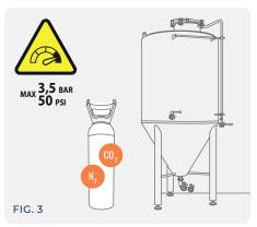
Check that the pressures of the filling system are correctly set and below the maximum value indicated. (3.5 bar/50 psi).
