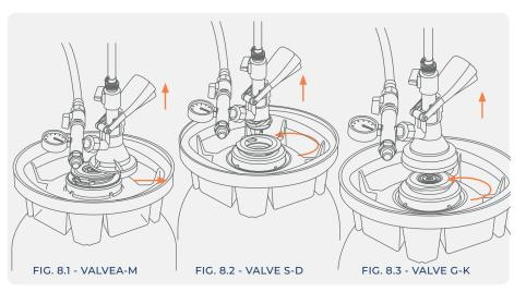
Quickly lift the lever and disconnect the coupler from the keg.
