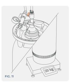
Once the nominal filling volume is reached, close the product valve. Do not exceed the nominal filling volume to prevent the product from leaking out of the bag.
