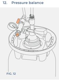
Close the regulator and work on the gas valve to increase the counter-pressure to a value slightly higher than the product filling value.
