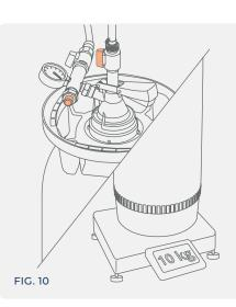
Open the product valve to start filling and work with the counterpressure regulator to set and/or change the filling speed.
