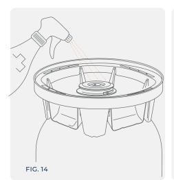
Remove any residual product with water, sanitize the external part of the valve as indicated in the "Sanitizing instructions" section and dry same.
