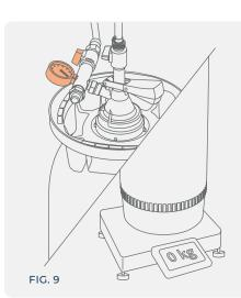
Work with the gas valve until the desired counter pressure is reached (approx. 0.5 bar lower than the product filling pressure).
